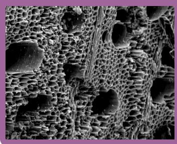
Biochar is **highly porous** and provides a permanent infrastructure for the **colonisation of beneficial micro-organisms** (as shown in the electron microscope image).
